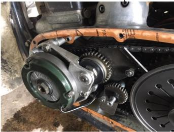
As many of you may know I bought my Mk3 new in 1976. For many years the electric start worked quite well and then I had a spate of sprag clutches failing (some of them only lasting half a dozen starts) so I removed the electric start, fitted a blanking plate and for many years I settled for just kicking the bike over.
